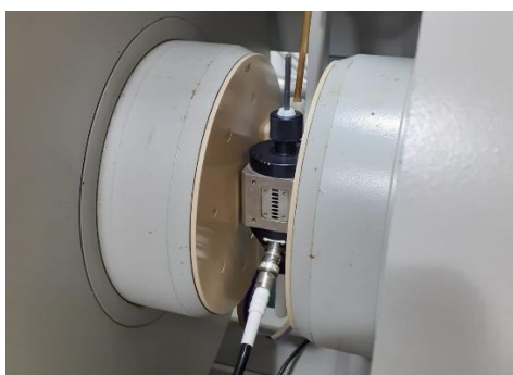
Figure 1: SLA-printed sample placed in the cavity of an EPR spectrometer.
